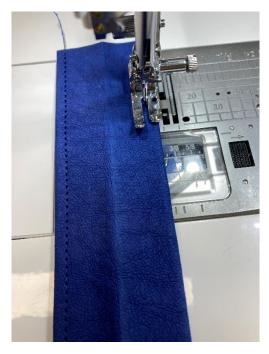
3. Fold strip back in half at the center crease, sew 1/4" tunnel at the fold to create a casing for the wire insert. Stop stitching and backstitch 1 ½" from each end. Take care when sewing through thicker parts of material to not break your needle.
